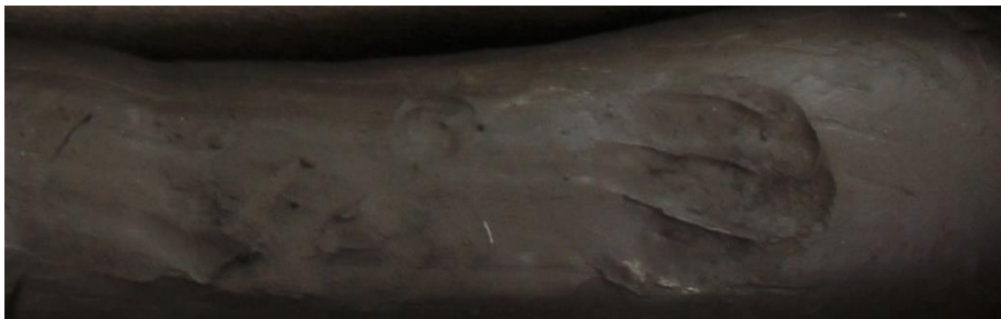
Tidal Flat Deposits Clay (c1), Soft thinly laminated dark brown slightly sandy silty CLAY with occasional fragments of white bivalve shell, MS\BH13 core run 4.20m – 5.70m.
