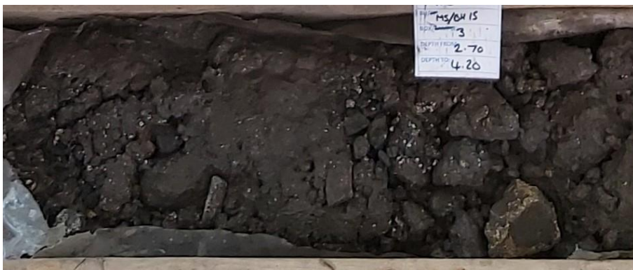
Granular Made Ground (d3), MADE GROUND: Grey slightly gravelly clayey fine to coarse SAND. Gravel angular to subrounded fine to coarse of various lithologies including slag, MS\BH15 core run 2.70m – 4.20m.
