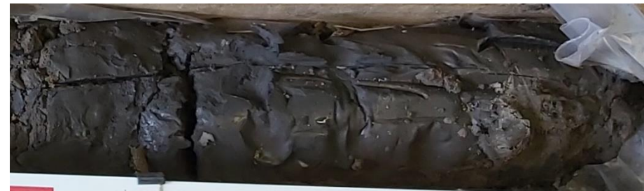
Tidal Flat Deposits Clay (c1), Soft grey and brown silty organic CLAY with frequent traces of organic material. Organic odour commonly noted, MS\BH10 core run 8.70m – 10.20m.
