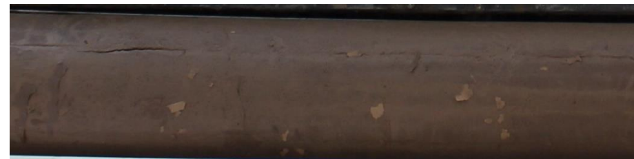
Tidal Flat Deposits Clay (c1), Soft grey and brown silty organic CLAY with frequent traces of organic material. Organic odour commonly noted, MS\BH10 core run 8.70m – 10.20m.
