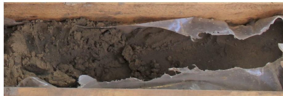
Cohesive Made Ground (d4), MADE GROUND: Soft to firm red brown and brown sandy slightly gravelly CLAY with low cobble content. Gravel is angular and subangular fine to coarse of various lithologies including slag. Cobbles are angular and subangular or slag and brick, MS\BH17 core run 1.20m – 2.70m.
