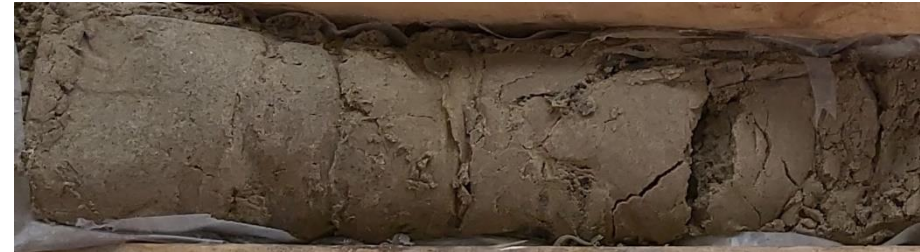
Tidal Flat Deposits Sand (c2), Medium dense yellow fine to coarse SAND with occasional fragments of white bivalve shell and pockets of soft brown silty clay, MS\BH16 core run 7.20m – 8.70m.
