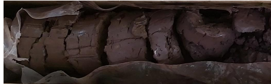
Cohesive Made Ground (d4), MADE GROUND: Soft to firm red brown and brown sandy slightly gravelly CLAY with low cobble content. Gravel is angular and subangular fine to coarse of various lithologies including slag. Cobbles are angular and subangular or slag and brick, MS\BH17 core run 1.20m – 2.70m.
